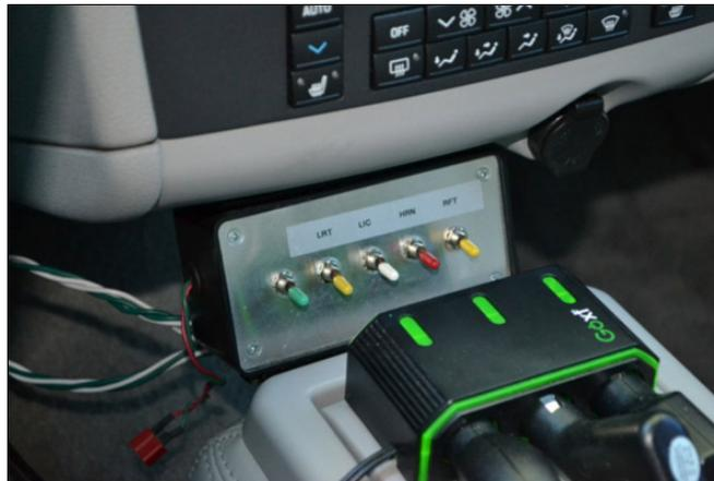
I installed a separate [12V power supply](#) and converter behind the driver's seat, so I have access to 120VAC and an additional [12V socket](#) so I don't have to suffer during those long stake outs. Now I can run my laptop, charge my cameras and not worry about running down my vehicle battery.
